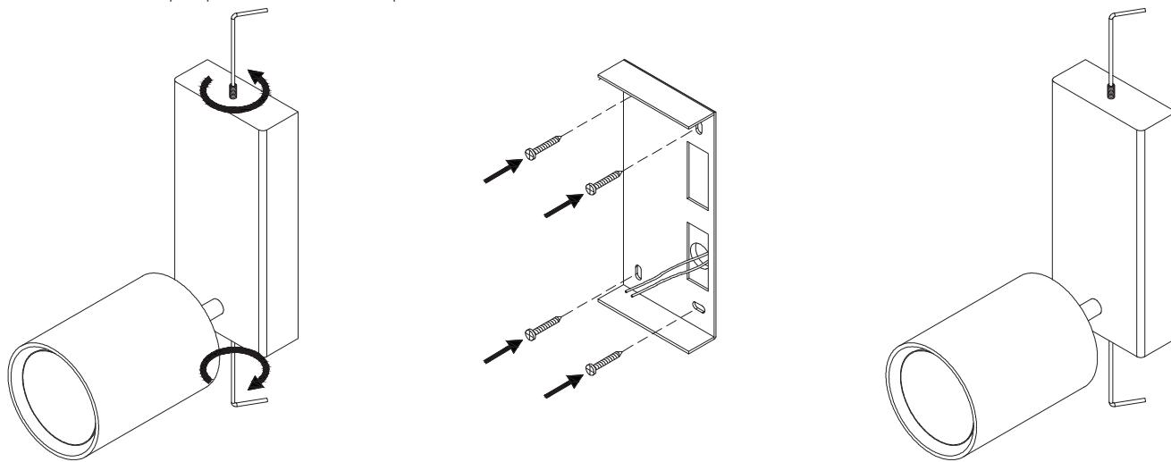
1 GB Loosen the fastening screws and remove the fastening bracket.
