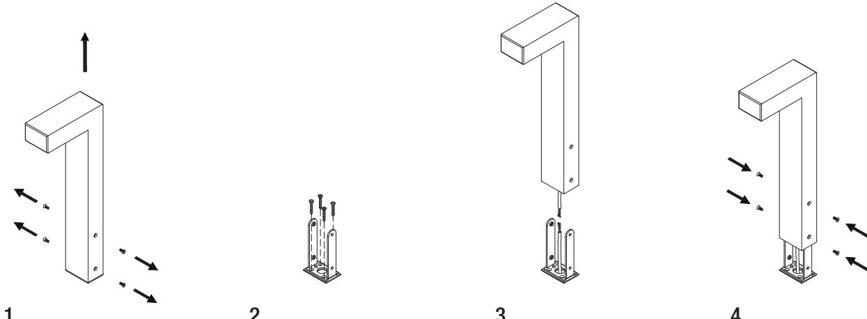
GB Remove the screws and extract the fastening bracket.
