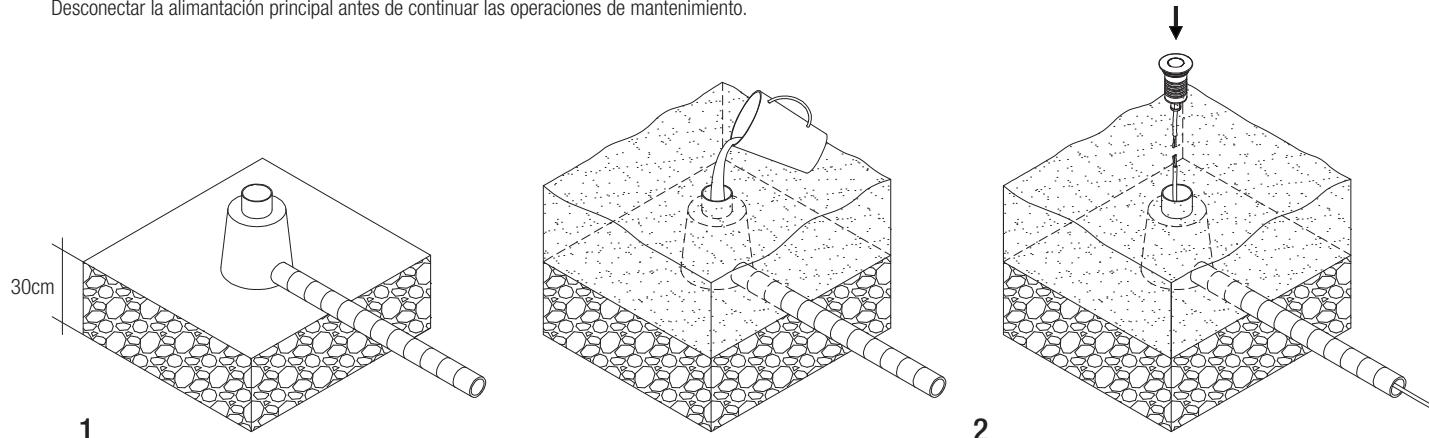
GB Prepare always 20-30 cm of drainage gravel and check that it works: fill the tube of water and check that it completely disappear within 30 min.
