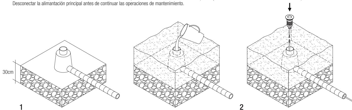
GB Prepare always 20-30 cm of drainage gravel and check that it works: fill the tube of water and check that it completely disappear within 30 min.
