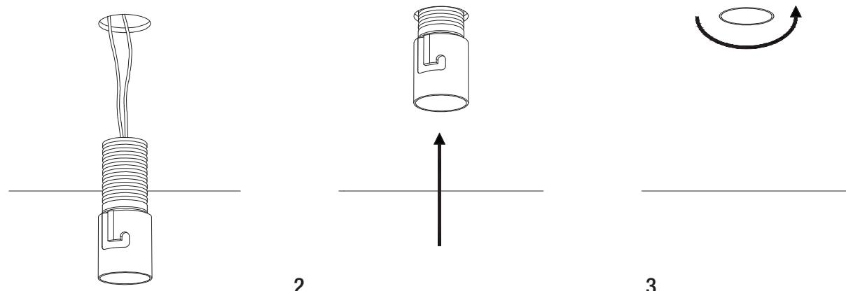
GB Install the electrical connections of the appliance to the power supply.
